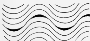
FIG. 49. Diagram to illustrate phacolith intruded in connection with folding. (After Harker.)
